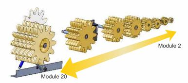
The gear lubricator segments are arranged onto a bushing. The bushing rotates around its mounting axle. The gear lubricator teeth meet precisely with the pinion drive teeth flank surfaces. A bore in the mounting axle supplies the lubricant to the gear lubricator outlets of the LUBCON LubeGearSystem.
